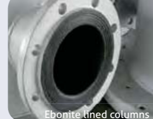
Ebonite lined columns
